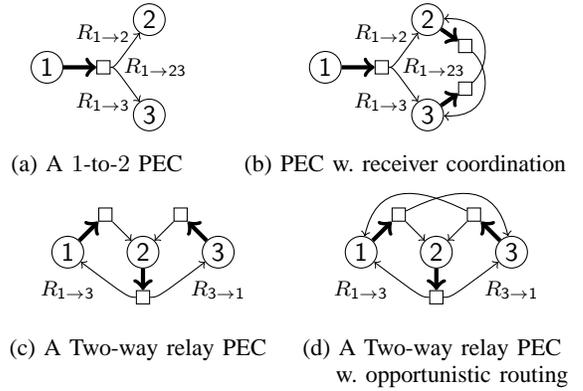
Fig. 2: Special examples of the 3-node Packet Erasure Network (PEN) considered in this work. The rectangle implies the broadcast packet erasure channel (PEC).
