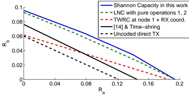
Fig. 3: Comparison of the capacity region with different achievable rates
